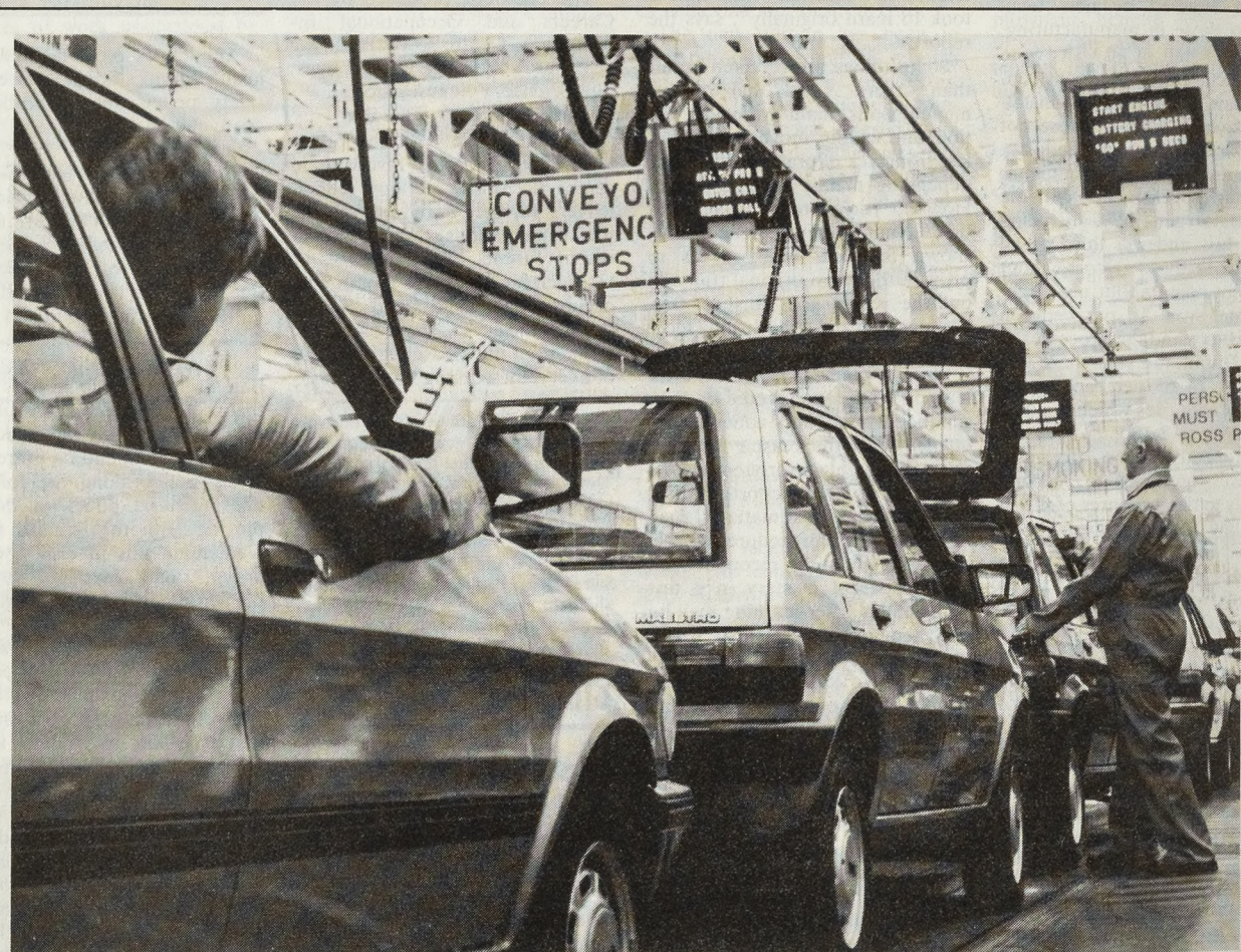
Austin Rover's vehicle electrical test system in operation to maintain Maestro quality.
