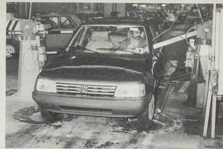
Automatic setting of the steering rack on the production line.
