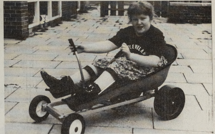
The prototype hand-propelled go-kart for paraplegic children, designed and built by apprentices from Cleveland Potash Ltd during their time at Cleveland Technical College, which came second in the class for 17 to 19-year-olds.
