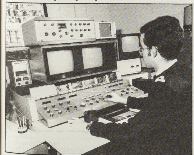
Final year degree student operating a scanning electron microscope at the Royal Naval Engineering College, Manadon.
