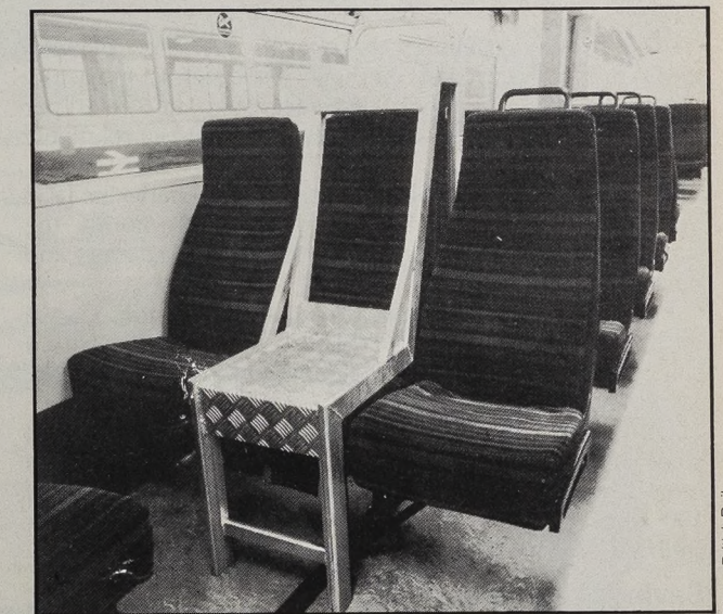
Carriage cleaners step ladder prototype designed by a British Rail Inspector.
